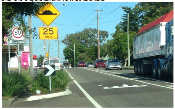
"The speed cushions are designed to provide the same impact on passenger vehicle motorists as a standard style speed hump, as the width of a car cannot straddle the hump and must still go over it.
